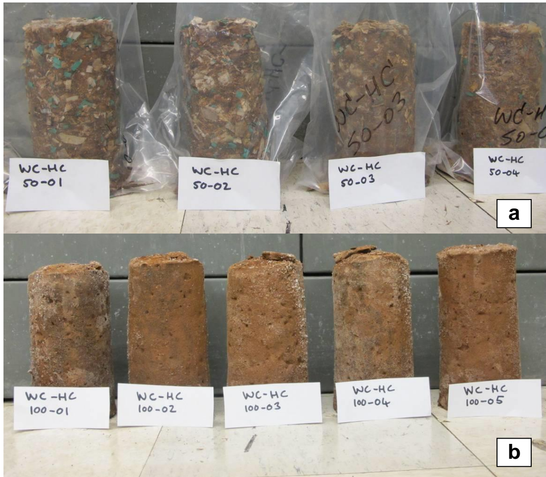
Figure 14. Post test 50% (a) and 100% (b) degraded hydrostatic compression samples.
