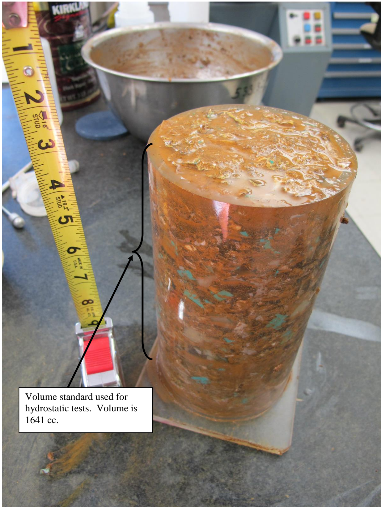
Figure 3. Saturated 50 % recipe contained within the 'volume standard' ready for insertion into gum rubber jacket assembly.
