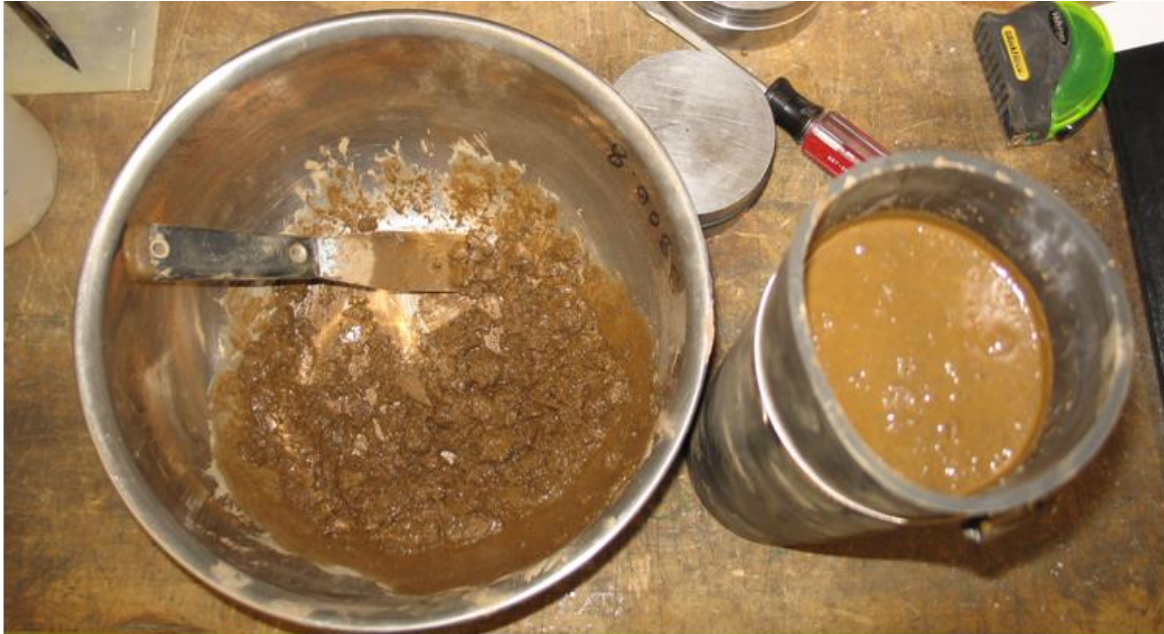
Figure 2. Batch of 100% degraded material ready for insertion into a sample mold.
